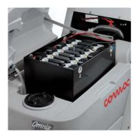
The battery compartment is positioned at the centre of the machine and it is integrated in the tank's volume. All around the batteries, the plastic materials are resistant to oxidising vapours so that any ugly and harmful rust formation is prevented
