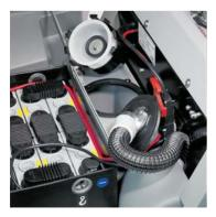
The suction motor is vertically positioned on the back. In the recovery tank area there is a clear division between the suction filter and the squeegee inlet whose shape has been designed in such a way to provide cyclonic performance effect of the air-flow. Without lifting the solution tank, the suction filter and the safety float can be removed for cleaning through the upper opening
