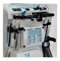
On the machine rear are the controls for lifting and adjusting the scrubbing head as well as the levers for service and parking brakes.
